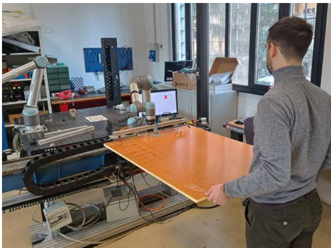
Fig. 1. The typical large object co-manipulation scenario. On one side, a lightweight robot is grasping a large object. The robot cannot hold the object alone because of a limited payload and workspace. Conversely, a human is grasping the same object, with possibly the same problems. In this situation, the robot can guide the human to approach with precision a target pose without exceeding its payload.
