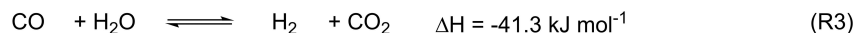
Scheme 1. Reaction network of methanol reforming including the side reaction (R2) leading to CO formation and the water-gas shift reaction (R3).
