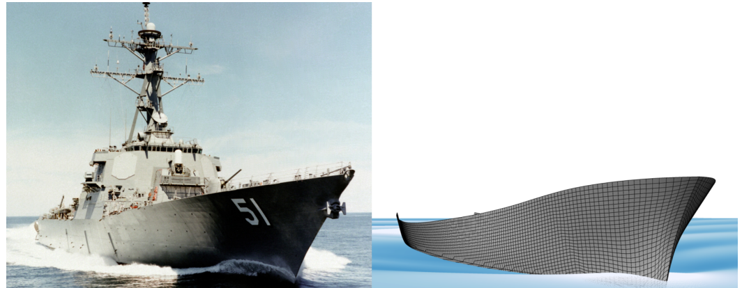
Figure 1. Starboard bow view of the Arleigh Burke-class guided missile destroyer (DDG-51, left) alongside its digital counterpart, the DTMB 5415 model (right).
