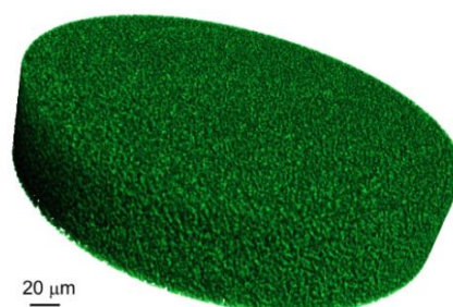
Figure 5. X-ray tomography 3D-reconstruction image of NbTiO-MNL2.
