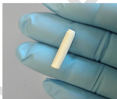
Figure 1. Optical image of dual porosity niobium-titanium oxide monolith.
