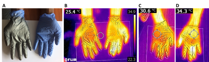
Figure 7. (A) Digital and (B) FLIR images of the uncoated and FLG-coated gloves, followed by a thermal treatment at 80 °C for 15 min. The experiments were carried out at an ambient temperature of 26 °C. The heat radiation can be clearly visualized on the FLG-coated glove which displays an orange thermal color (left) instead of a bright-yellow color for the uncoated one (right). (C) FLIR image of FLG@glove and (D) uncoated glove with almost 4 °C difference in terms of heat radiation.
