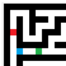
Fig. 5 State [(10; 10; 0)_#FFFFFF, (5; 7; 0)_#FFFFFF, Driver, Close] of the composition of two agents, a driver, and a door. The door is in position (2; 7) and is closed. The first agent is depicted red, the second is green, and the door is blue. The attributes of the position of the two agents are both #FFFFFF, which is the hexadecimal value for the colour white, i.e., both agents are placed on a white cell of the map.
