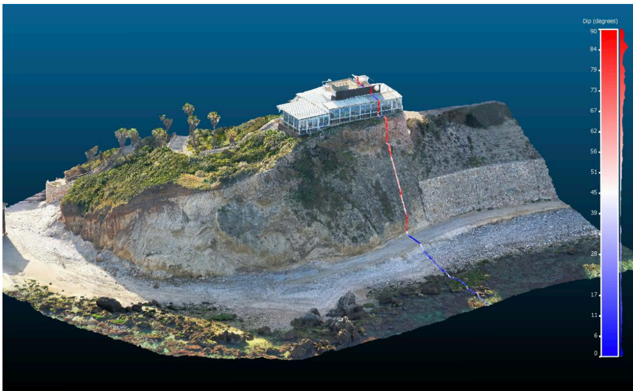
A 3D model of the Bet Hankin restaurant on the shoreline cliff at Hadera, Israel. The red-blue scale represents the slope (degrees) on the reference section marked. A colour-code for the slope is given on the right, together with a histogram (principal mode 85°).
