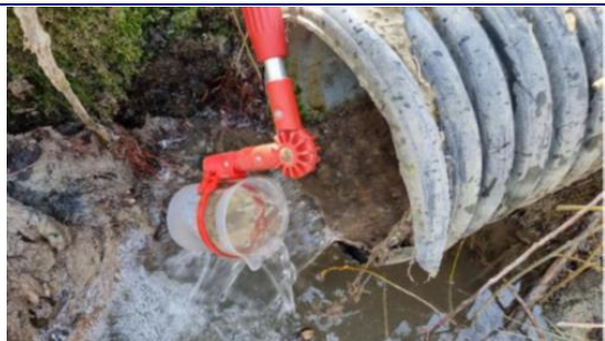
Figure 1 – wastewater sampling phase
