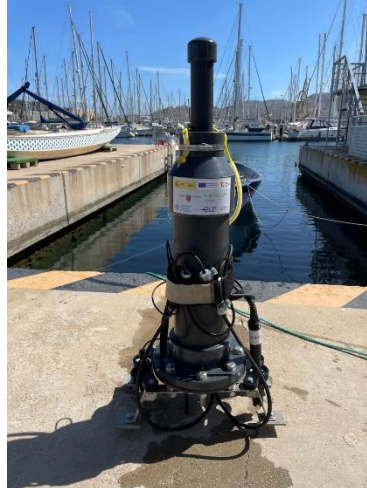
Figure 1. \mu -Nautilus prototype with integrated sensors.
