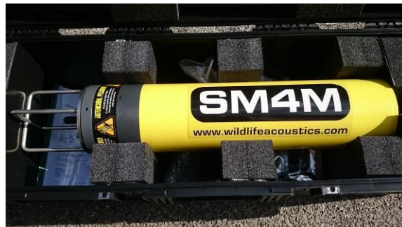
Fig. 2. Wildlife Acoustics SM4M autonomous recorder calibrated within the UNAC-LOW project.
