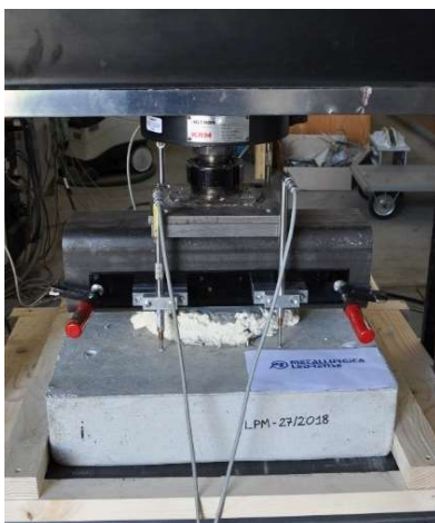
Figure 6. Hinge connection at the end of the test: compression (left) tensile (centre) and shear (right)
