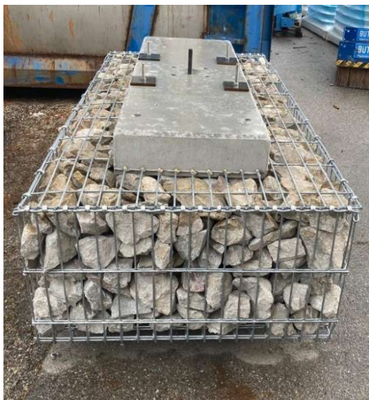
Figure 1. The welded mesh gabion box filled with aggregates (left) and the hinge connection (right)
