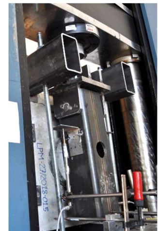
Figure 6. Hinge connection at the end of the test: compression (left) tensile (centre) and shear (right)
