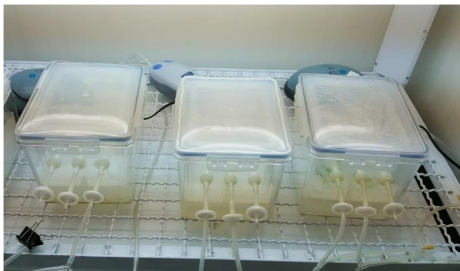
Figure 1. PlantForm bioreactor TIS model consisting of one container.
