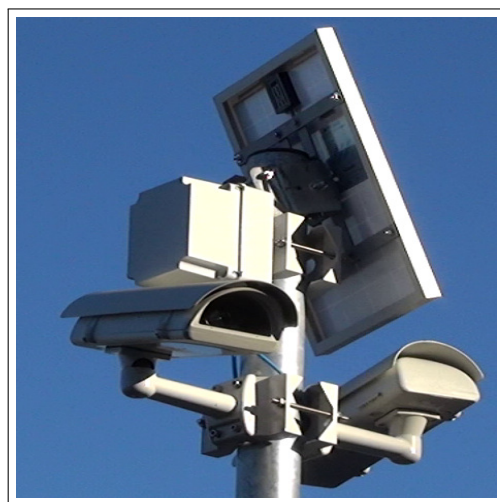
Fig. 3. An installed prototype with two complete sensor nodes
