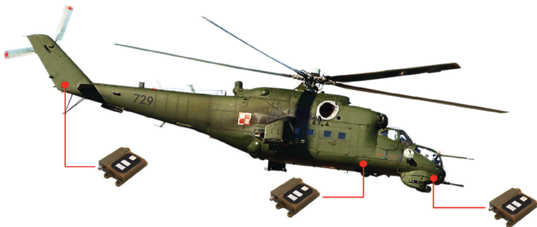
Figure 1. CHM system consisting of three autonomous sensors installed on in-service Mi-24
