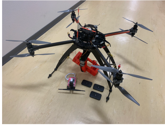
Fig. 2: The testbed platform in use: a custom UAV, an RPi equipped with a camera, and three 4G modems.
