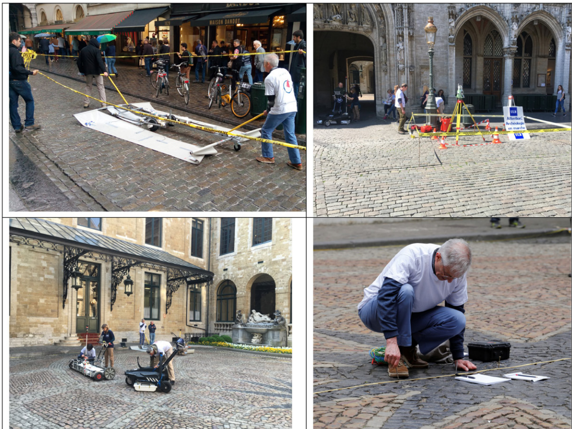
Figure 2. MP3 prototype for measuring apparent resistivity, operators (A. Tabbagh and S. Flageul) are within a ‘moving’ safety zone delimited by yellow tape; Robotic total Station operated by B. van Nieuwenhoeve; GPR (StreamC 600 MHz and StreamX 200 MHz, IDS GeoRadar Corporation) G. Morelli and G. Catanzariti; Vertical electrical Sounding between the cobblestones in the Townhall (A. Tabbagh).
