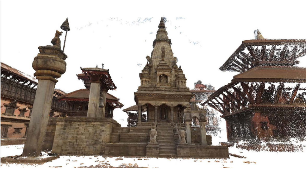
Figure 3. The Vatsala Durga temple (Bhaktapur Durbar Square, Nepal) as reconstructed from old photographs.
