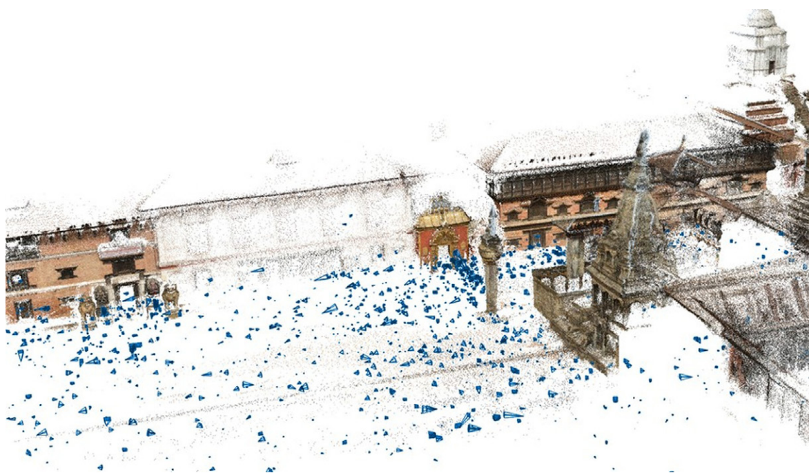
Figure 2. Bhaktapur Durbar Square, Nepal. Point cloud reconstructed from many images (blue triangles). The Vatsala temple is seen on the right.
