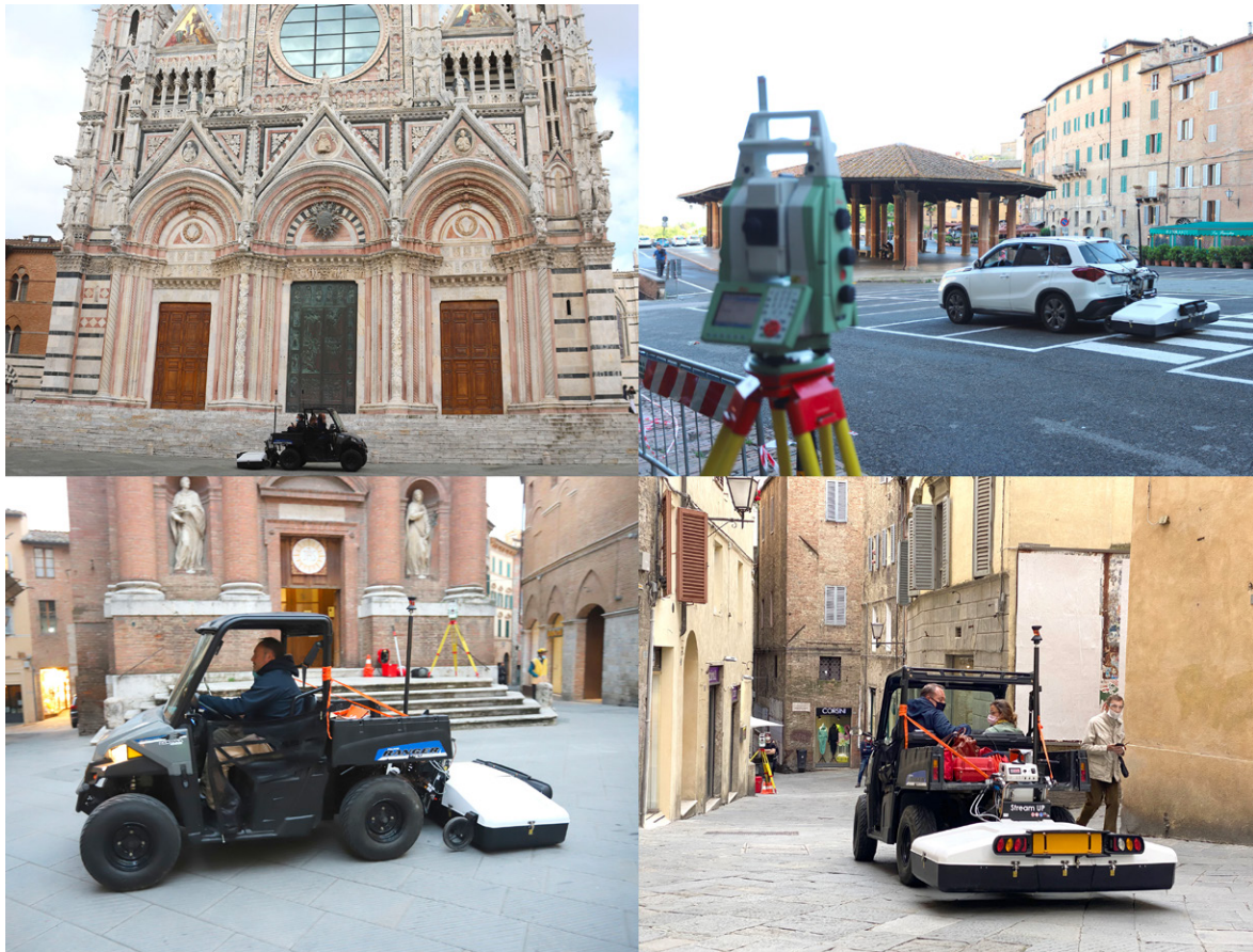
Figure 2. Survey activities by IDS STREAM UP radar system.
