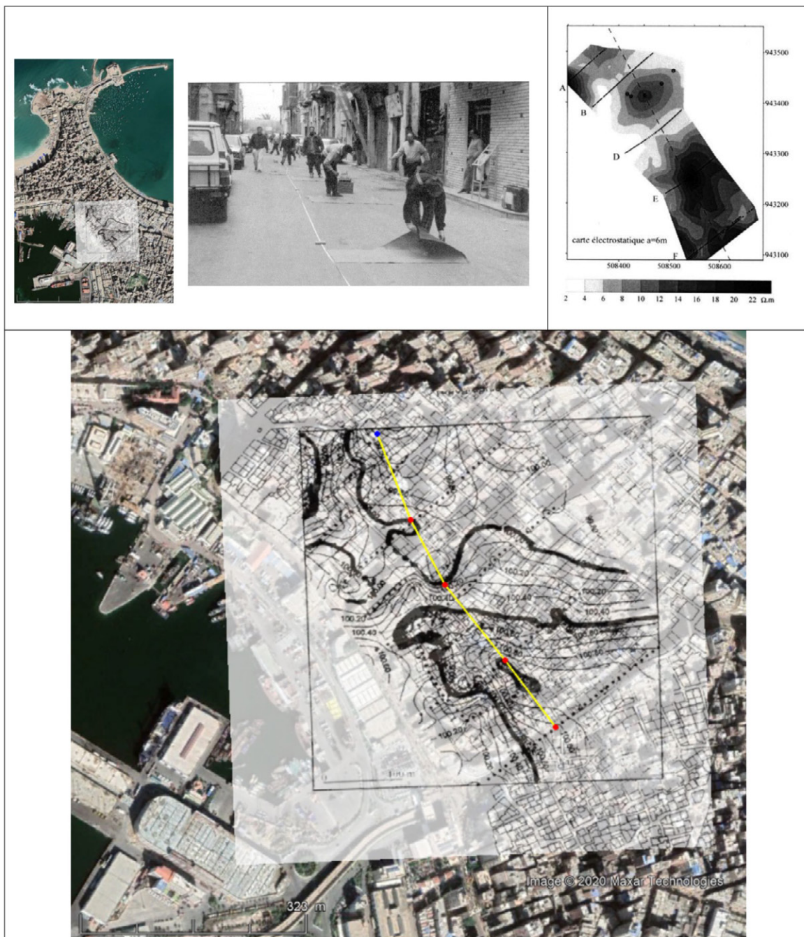
Figure 1. (from top to bottom, clockwise): Position of the geophysical surveys in Alexandria (white square); Electrical Profiling using independent electrostatic quadrupoles in Wenner configuration ( a=6 m) along one of the streets (credit: A. Hesse); Map of apparent electrical resistivities obtained by krigging the data along the 6 profiles (Hesse et al. , 2002); Superposition of microtopography and Google Earth showing in yellow the proposed causeway for the Heptastadium (credit: A. Hesse, M. Dabas).
