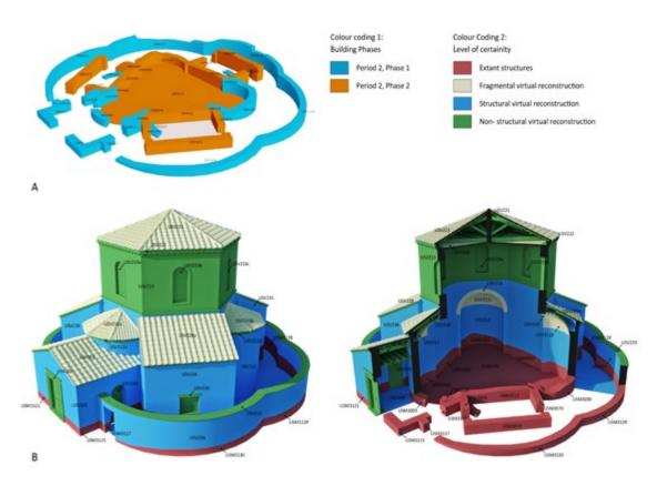
Fig. 10. A) proxy model highlighting building phases; B) proxy models highlighting level of certainty.
