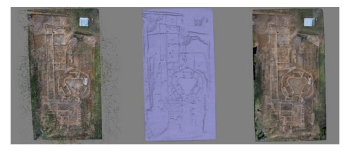
Fig. 4. Data processing in Photoscan. Dense point cloud computation through DSM algorithms; Solid mesh model obtained by point triangulation; Textured model by projection of images.
