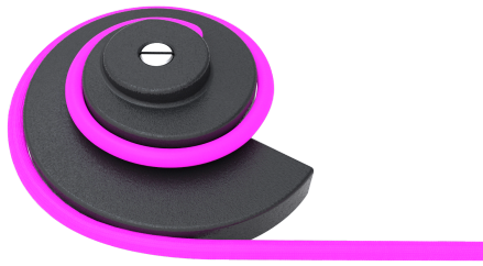
Figure 21: A multiple-turns spiral cam can increase the exploitable wire stroke reducing the overall dimensions of the cam.
