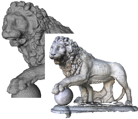
Figure 1: Image from a 3D model obtained with passive reconstruction from a set of digital images (by ARC 3D and MeshLab tools).
