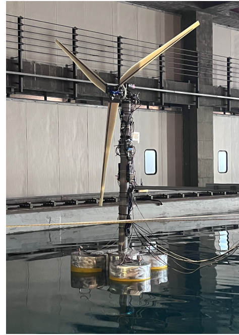
(a) Schematic of the hybrid platform and its main components (b) A photograph of the physical device deployed in the towing tank
