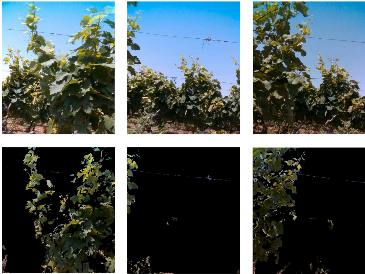
Fig. 13. Image sequence in proximity of position P3: original color images (up) and depth-based segmented images (bottom). In this case, depth-based segmentation points out a region with low foliage occupation (plants on the background are filtered out based on distance information). Hence, the system can simultaneously capture appearance and morphological characteristics of the crop, based on RGB-NIR and depth data, respectively.
