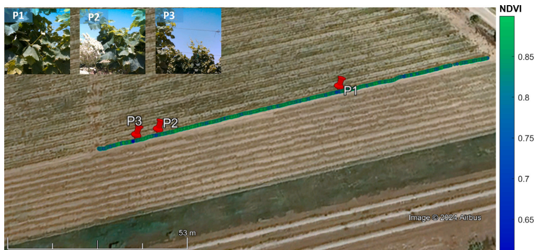
Fig. 12. Google Earth projection of NDVI measurements (displayed in winter color map) along row 1 inspected from side B, with greener points denoting higher NDVI values. Attention spots (points with lower NDVI such as P1, P2, P3) can be easily detected and the corresponding images retrieved for further inspection.
