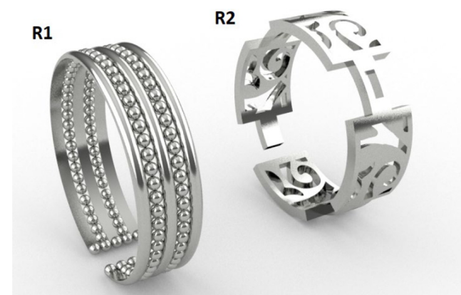
Figure 5 3D CAD model of R1 and R2 opened rings
