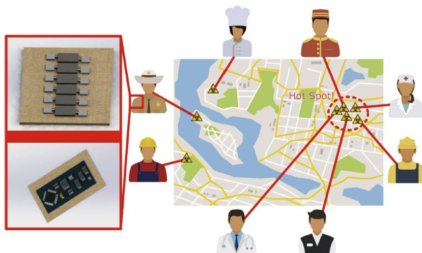
Fig. 2. Schematic of envisioned application space for the GO screen printed flexible impedance biosensors. Sensors arrays implemented on textiles and interfaced with flexible electronics can report the location of positives and identify sources of the outbreak. Reproduced with permission from [35], Creative Commons. Printed with permission from IOP Publishing.
