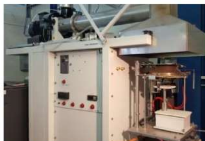
Figure 1: Bomb calorimeter for testing according to EN ISO 1716 (left) and test apparatus for testing according to ISO 5660-1 (right)
