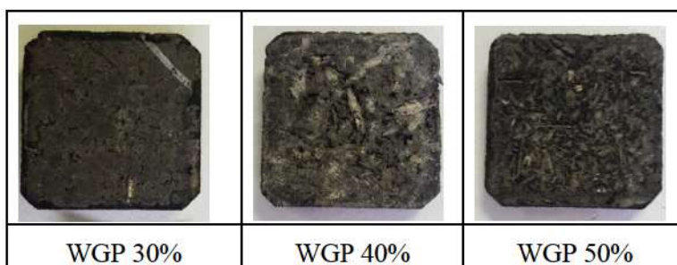
Figure 6: Photos of the three tested materials after the test with cone calorimeter method (ISO 5660-1) at 50 kW/m 2 of heat flux
