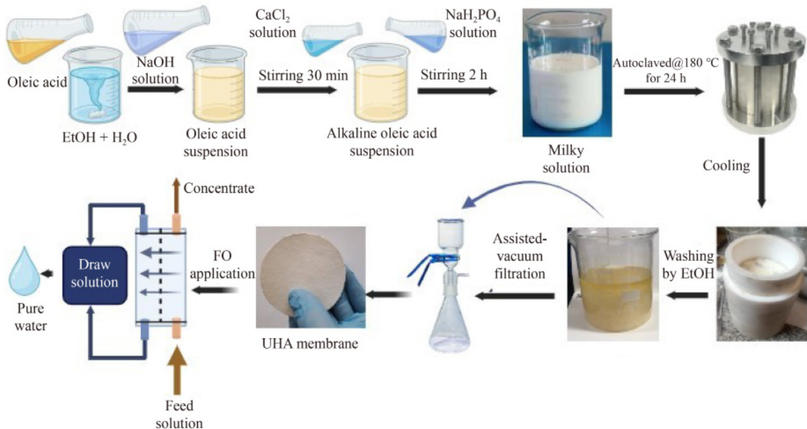
Fig. 1 Preparation of the UHA membrane.
