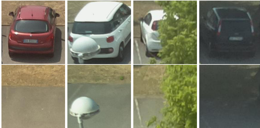
FIGURE 3: TRAINING SET PATCHES SEGMENTED FROM THE CAMERA VIEW. IMAGES SHOW FOUR PARKING SPACES IN BOTH STATUS: BUSY (FIRST ROW) AND FREE (SECOND ROW). THEY ALSO PRESENT SOME OCCLUSION AND SHADOW SITUATIONS THAT WE FACED.
