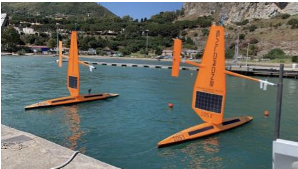
Figure 4: SDs in Cefalù, where they stayed anchored due to low wind speed and where also biofouling and fishing gears were removed from the drone's hull.
