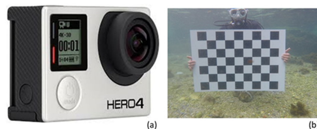
Figure 4. (a) GoPro HERO 4 Black camera used for seafloor mapping. (b) Example of underwater image of the chessboard used for camera calibration.
