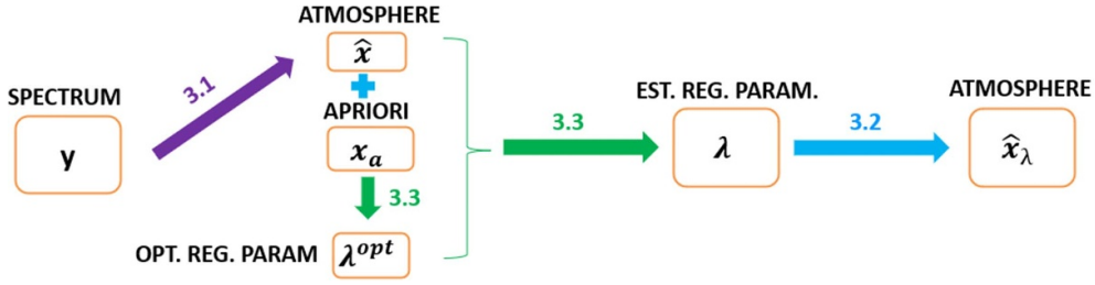
Figure 2. Solution scheme where the different steps are represented with arrows of different colors with the related section indication: purple for data-driven step, blue for regularization step and green for regularization parameters computation and estimation.
