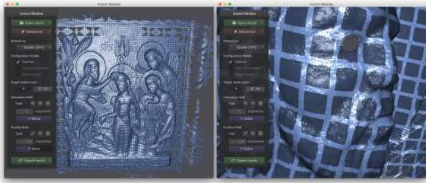
Figure 15: Screen captures of a point cloud meshing session conducted using our interactive implementation
