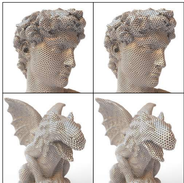
Figure 16: Triangle meshing comparison: [Surazhsky et al. 2003] (top left), [Pietroni et al. ] (bottom left) and our results on the right. Note that our meshes are better aligned to the shape features.
