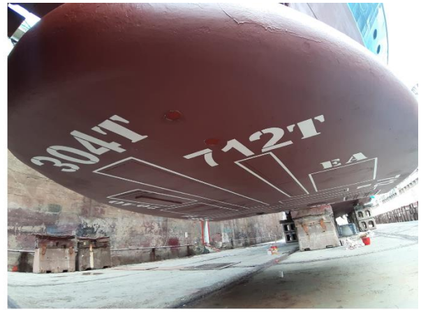
Figure 21 - Keel-mounted installation of EM2040 and EM712 MBES systems on GAIA BLU N/R (left: starboard side, right: port side). Photo credit: Giovanni De Vita, Argo S.r.l.
