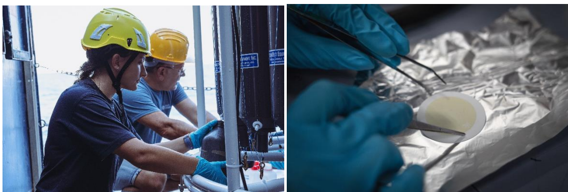
Figure 13 - Water sampling operations and filtration in the wet lab for eDNA analysis
