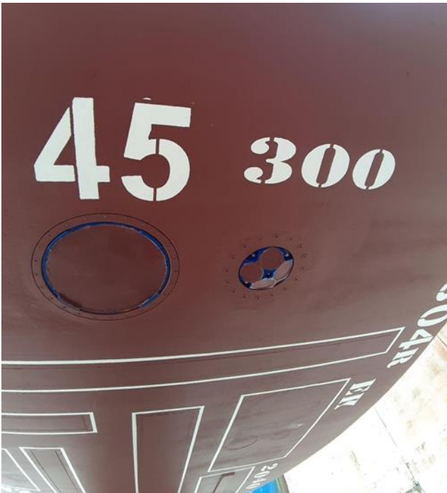
Figure 11 - Mounting locations of the two vessel-mounted ADCPs, the Pinnacle 45 kHz and the Workhorse Mariner 300 kHz, on the hull of the R/V Gaia Blu. Photo provided by Giovanni De Vita, Argo S.r.l.
