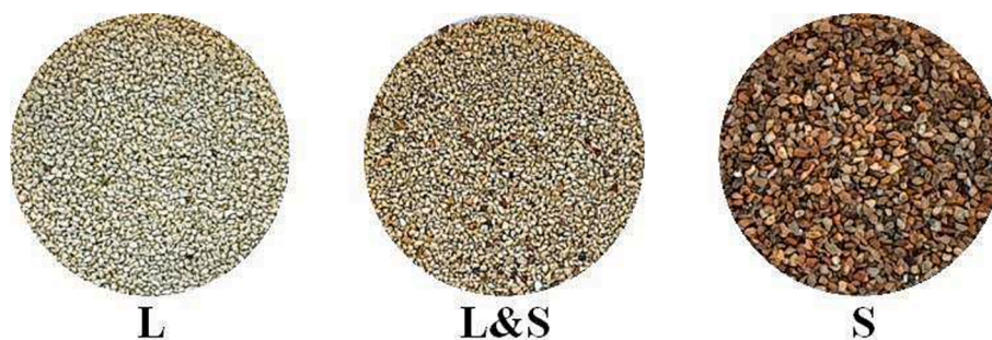
Fig. 11. Picture of: lime samples retrieved after the last calcination step in the electrically heated FB, for tests performed with a bed inventory of limestone only (L) and limestone and sand (L&S); pure sand (S).
