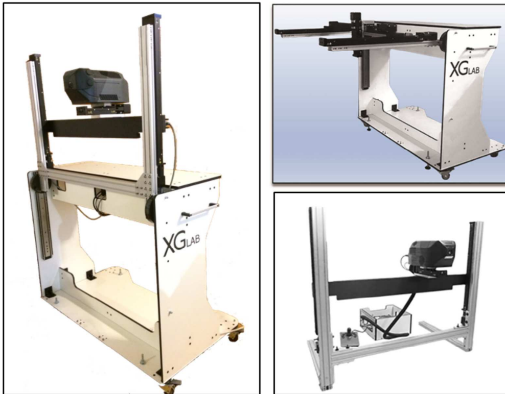
Fig.1: Crono XRF detection head mounted on the motorized frame and trolley in some of the possible configurations (vertical, horizontal, only the frame on the floor).
