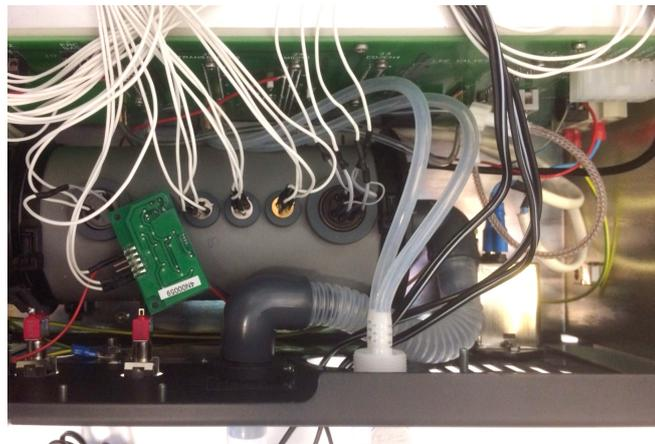
**Figure 4.15:** *First prototype of the sampling chamber with gas sensor array.*
