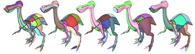
Fig. 7. Left-most: original mesh \mathcal{M} color-coded according to the quads in \mathcal{Q} (left). Then: examples of different assemblages of macro-regions. Triangles of \mathcal{M} which span multiple macro-regions (which are frozen during relaxation) are shown darkened.
