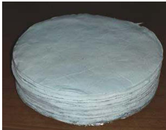
Figure 1. Layers of electrospun silica/PVP blanket.
