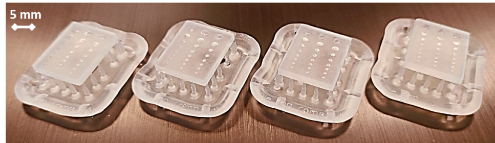
Figure 12. A picture of the four samples with variable compensation. Each sample has three patterns of sub-mm cavities with varying diameters, from 2 mm down to 500 μm.
