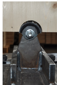
Figure 6. FIT failure modes RADIAL60D/S: embedment (left), screws withdrawal (centre) and bolt shear failure (right)
