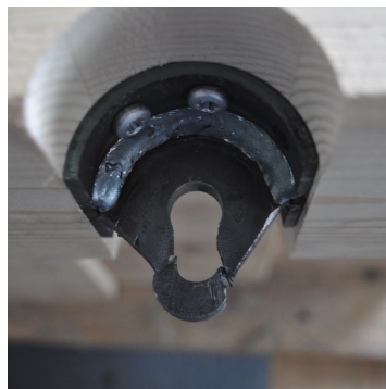
Figure 6. FIT failure modes RADIAL60D/S: embedment (left), screws withdrawal (centre) and bolt shear failure (right)
