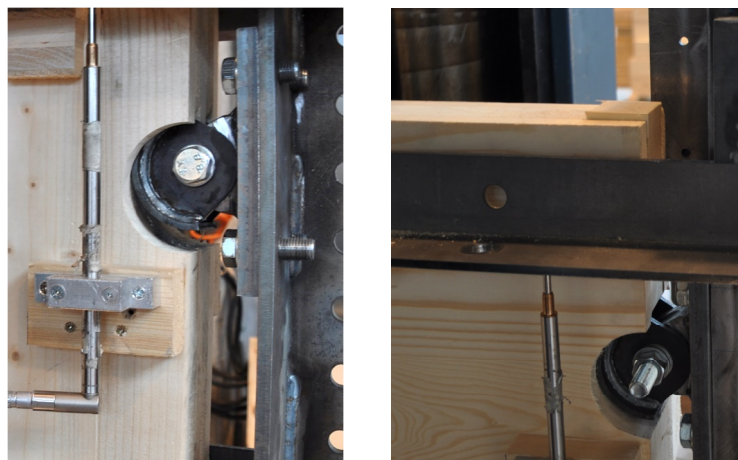
Figure 8. F2/3 failure modes RADIAL90: screw tensile (left) and CLT panel shear failure mode (right)
