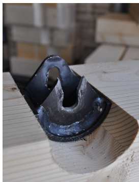
Figure 6. FIT failure modes RADIAL60D/S: embedment (left), screws withdrawal (centre) and bolt shear failure (right)
