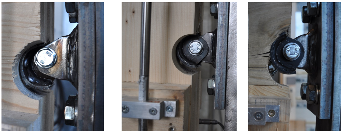
Figure 9. F2/3 failure modes RADIAL60D/S: screw tensile 60S (left), screw tensile 60D (centre) and screws withdrawal 60D (right)
