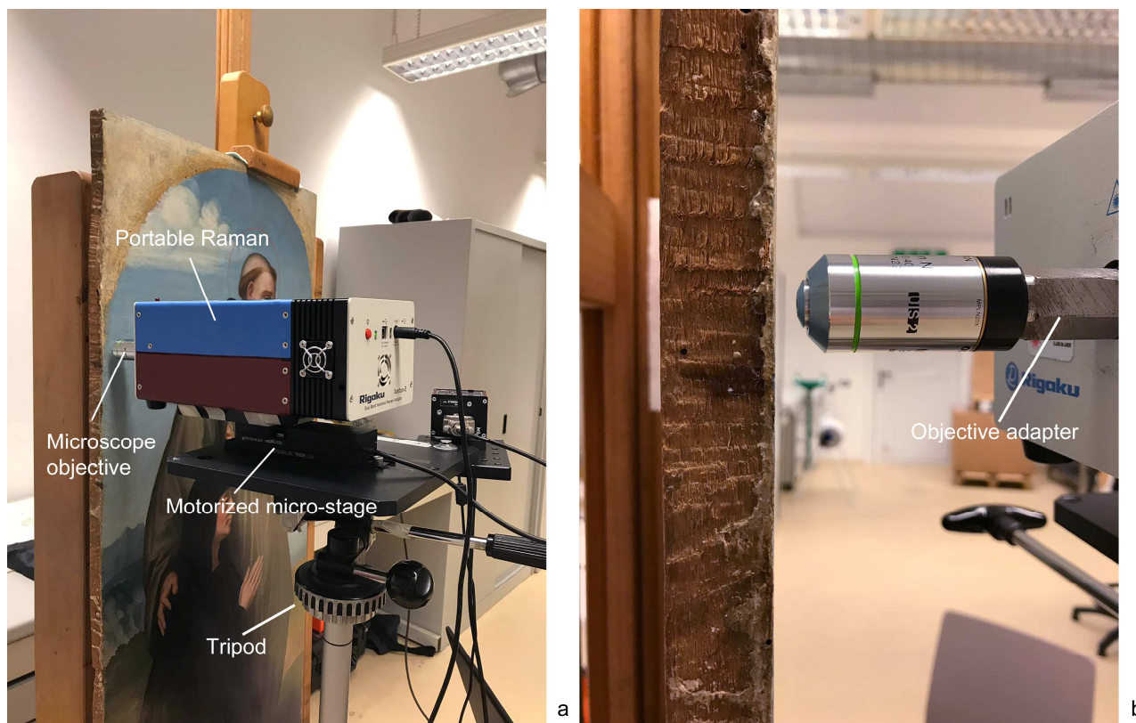
Figure 2: (a) portable Raman device optimised for micro-SORS measurements; (b) detail of the microscope objective and its adapter.
