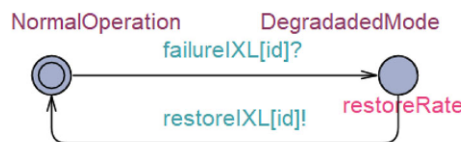
Fig. 20. The IXL_Mitigation automaton
