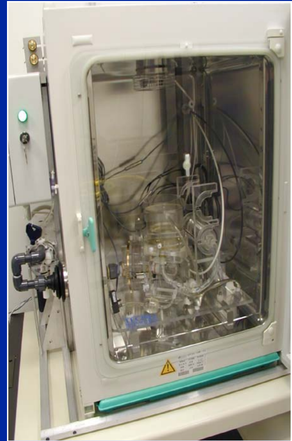
Bioreactor located into a standard CO 2 incubator
