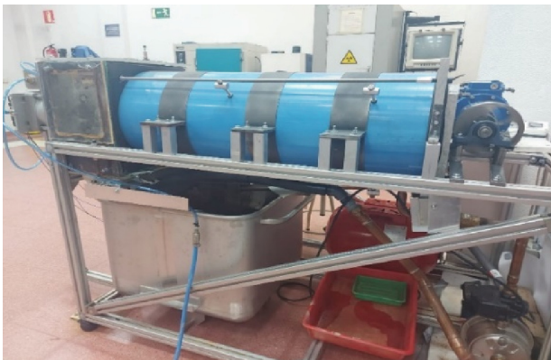
Fig. 1. Slamming Playback Equipment with built-in eccentric cam
