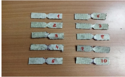
Fig. 10. Specimens used in the shear test
