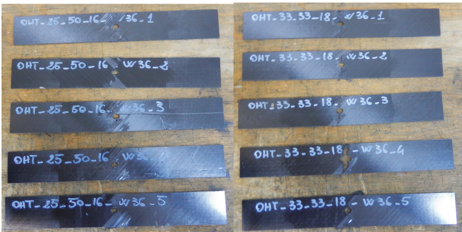
Fig. 4. Failed specimens OHT1_1, OHT2_1 (from left to right).
