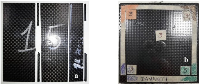
Fig. 3. Both laminates are with 15 plies, for [a] was used 30 min and [b] 60 min in the press machine
