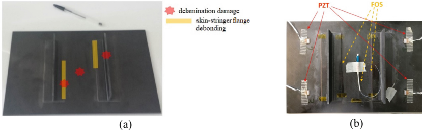
Fig. 3. Small stiffened panel, 350 mm \times 230 mm: (a) damage scenario; (b) SHM system.
