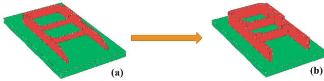
Fig. 5. First design idea (a): the designed component we want to obtain; deposition (b): redesigned component to take into account over metal compensation for post – processing machining.
