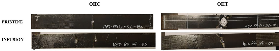
Fig. 2. Failure mode OHC and OHT tests
