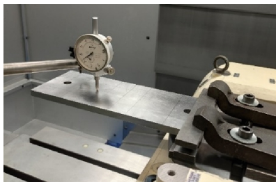
Fig. 9. Comparator setup with the clamped substrate.
