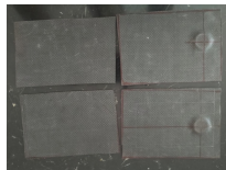
Fig. 3. Laminated specimens with (right) and without (left) the embedded Teflon layer.
