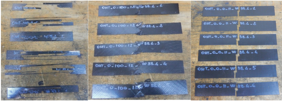
Fig. 3. Failed specimens OHT0, OHT45, OHT90 (from left to right).
