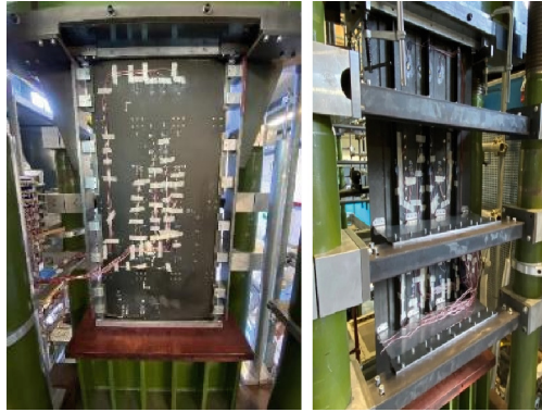
Fig. 6. Test set up completed and ready to start fatigue cycling.
