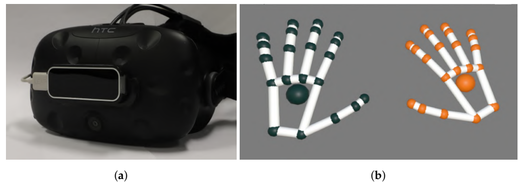
Figure 6. (a) Leap Motion device mounted in front of the helmet of the HTC Vive. (b) Stylized model of the hands tracked by the Leap Motion.
