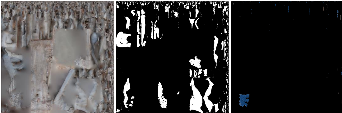
Fig. 10. Creation of masks to overlap different layers of colour: original colour (left); preparation of mask (centre); blue colour mask (right).
