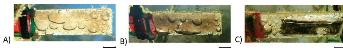
Figure 5. Pictures acquired at day 10 of immersion relative with different surface roughness: (A) Sa = 1.67 \mu\text{m} , (B) Sa = 1.95 \mu\text{m} , (C) Sa = 2.92 \mu\text{m} . Scale bar under each sample is 10 mm.
