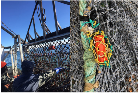
FIGURE 1 | Left: A temperature and depth sensor on a scallop dredge in the Gulf of Maine. Image: Cooper Van Vranken. Right: A sensor on a trawl net headrope, Aleutian Islands, Alaska. Image: Lynn Selboe. Sensors: NKE Instrumentation.
