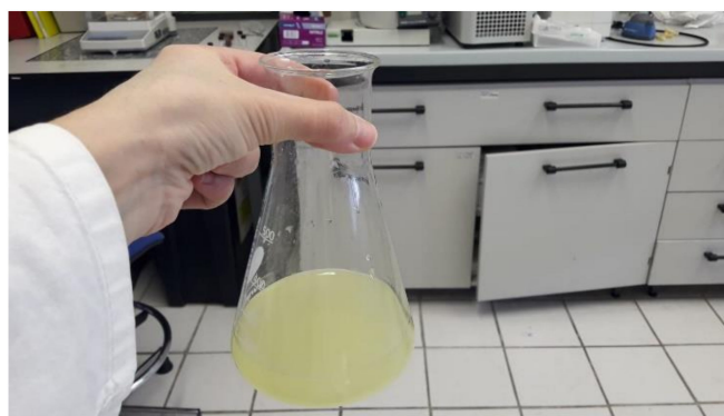
Figure 4. The yellow aqueous solution following hydrodynamic cavitation of waste lemon peel (image courtesy of Dr. M. Pagliaro, CNR).
