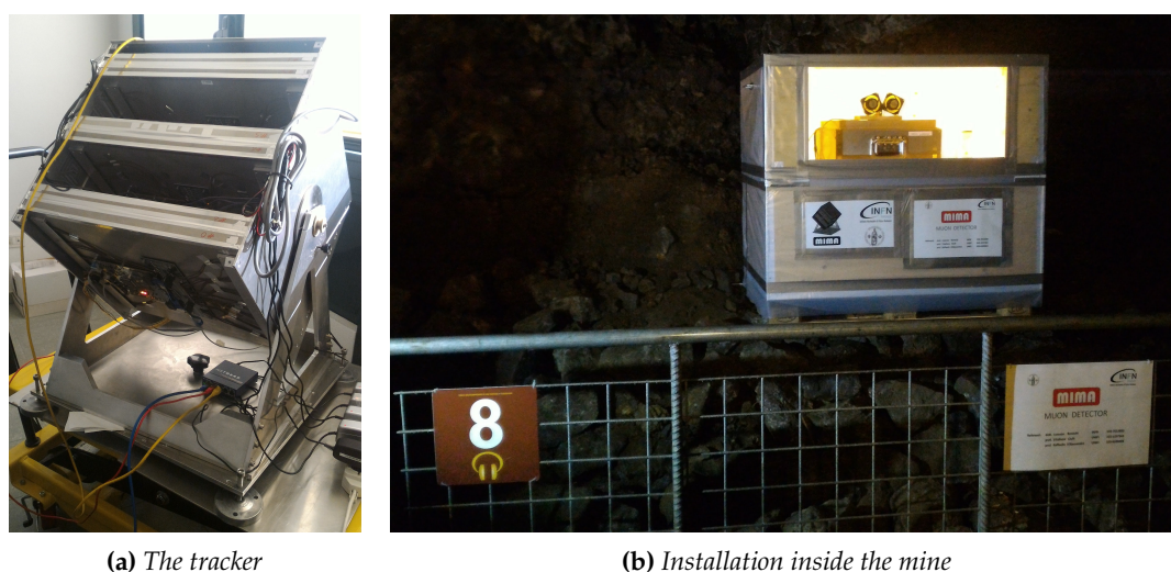
Figure 1. (a) Structure of the MIMA detector: we can see the three X-Y tracking modules, the rotating platform and part of the electronics. (b) A picture of the installation inside the Temperino mine. In this case the detector was placed inside a wooden box and it was equipped with an incandescent lamp and two small fans to protect it against moisture.
