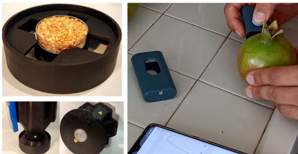
Fig. 1 The Phasmafood multisensor prototype (left side, top and bottom pictures) and SCiO spectrometer (right side) with the respective samples (cereals and pomegranate)
