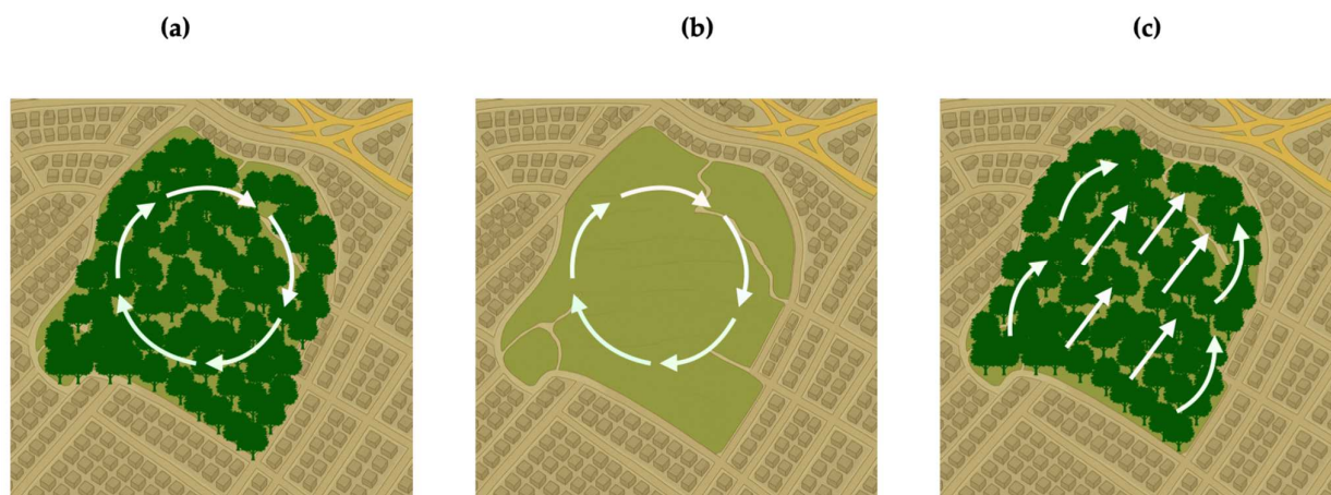
Figure 3. Schematic representations of the three simulation scenarios: (a) Scenario 1, with current tree cover under heatwave conditions and stagnant air flow; (b) Scenario 2, same meteorological forcing as (a), but with trees replaced by short grass; (c) Scenario 3, same vegetation as (a), but under enhanced ventilation conditions following a rainfall episode. White arrows represent idealized wind circulation over the park.
