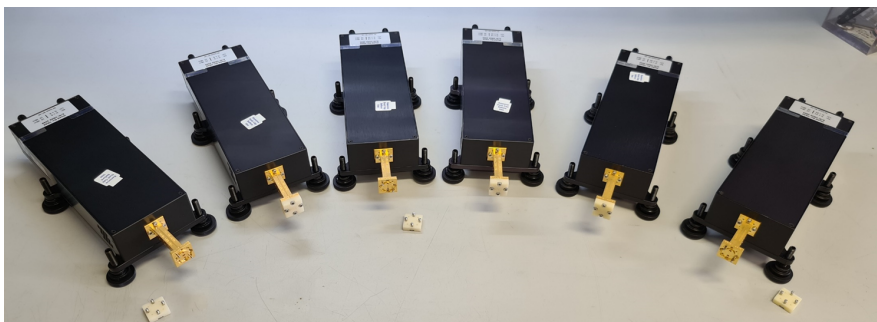
Figure IEIIT2: Millimetre wave/subTHz extenders operating at W-band (65-115 GHz), G-band (170-260 GHz) and 500-750 GHz.
