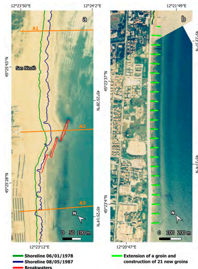
Figure 6. Coastal structures: (a) cell A, silting up of two breakwaters; (b) cell B, extension of the groin at the northern end of the Murazzi (in red), and construction of 21 new groins (in green) placed at a regular distance (aerial photographs taken in 1987; source: Regione Veneto). Orange lines (i.e., A1 to A3): transects.
