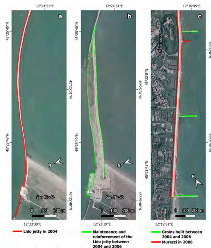
Figure 7. Coastal structures: (a) cell A, maintenance and reinforcement works at the jetty of Lido (in red) as a part of the realisation of the MoSE structures (2004 MAV); (b) the reinforcement works (in green) of the jetty occupied part of the dune surface and the beach of San Nicolò (aerial photographs taken in 2006; source: MAV); (c) cell B, 3 new groins (in green) equidistant between Malamocco village and the southern end of the Murazzi and reinforcement works (in red) of the Murazzi (aerial photographs taken in 2004; source: MAV).
