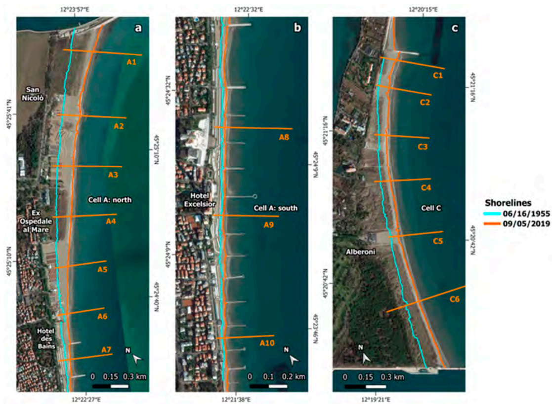
Figure 12. Shoreline changes between 1955 and 2019 from north to south; (a,b) cells A; (c) cell C (ESRI 2022, acquired through HCMGIS plugin for QGIS). Orange lines (i.e., A1 to A10 and C1 to C6): transects.
